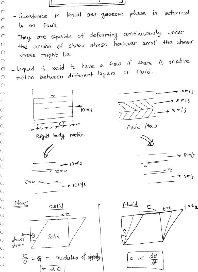
In cone of solid, shear stress is proportional to shear strain but in case of fluid shear stress is proportional to shear straim rate.
