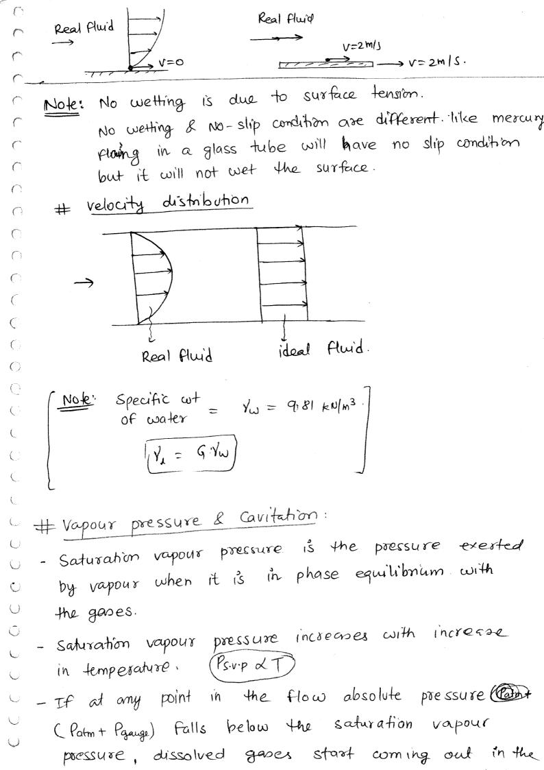
form of bubble creating cavity in the flow. These bubble travel due to momentum of flowing fluid and when it reaches the high pressure zone the bubble collapses giving rise to high pressure waves which causes noise, vibration, surface pitting and fatigue
